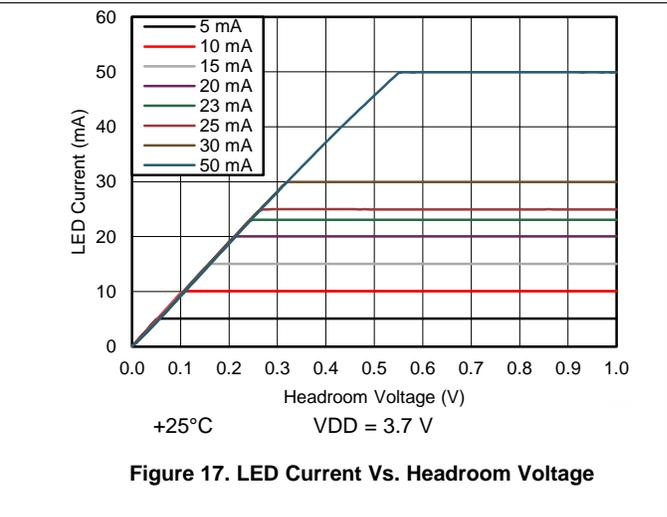
**Figure 17. LED Current Vs. Headroom Voltage**
