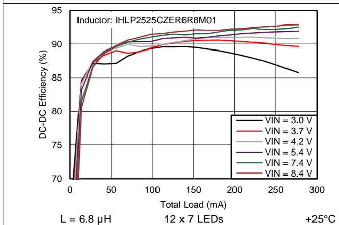
Figure 4. Boost Efficiency
