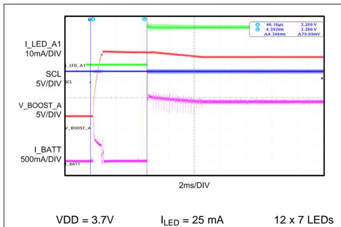
**Figure 45. Start-up Waveform with I<sup>2</sup>C Write Full Brightness Slope Function Disabled.**
