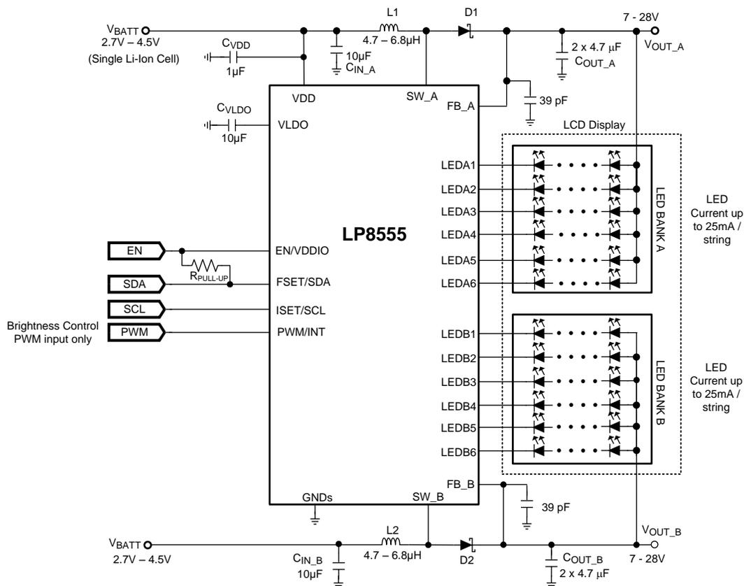
Figure 43. Application Diagram for Default EPROM Setup
