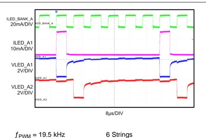
**Figure 48. Typical LED Current and Voltage Waveforms.**
