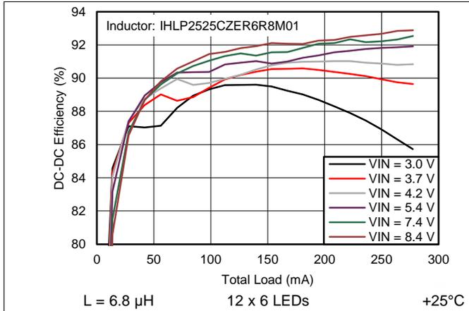
Figure 2. Boost Efficiency
