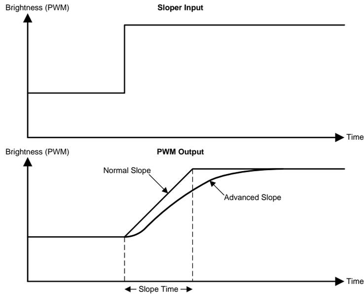
**Figure 32. Sloping Principle**
