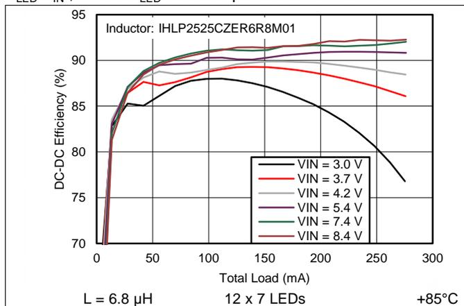
Figure 8. Boost Efficiency
