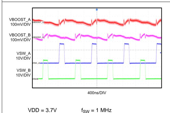
**Figure 47. 180° Phase Difference Between Boost A and B**
