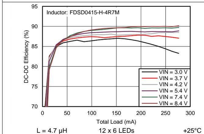
Figure 10. Boost Efficiency
