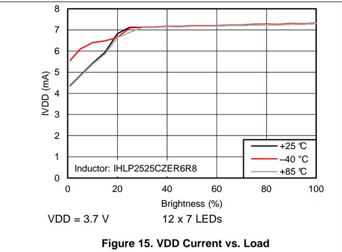
**Figure 15. VDD Current vs. Load**
