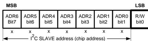
Figure 40. I<sup>2</sup>C Slave Address
