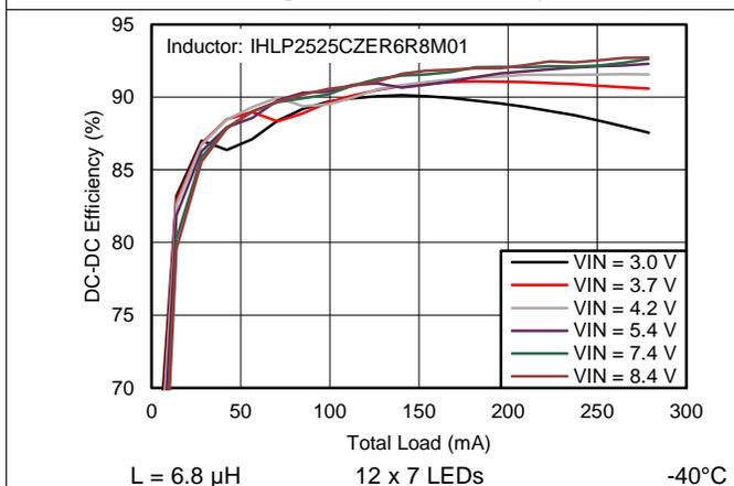
Figure 6. Boost Efficiency
