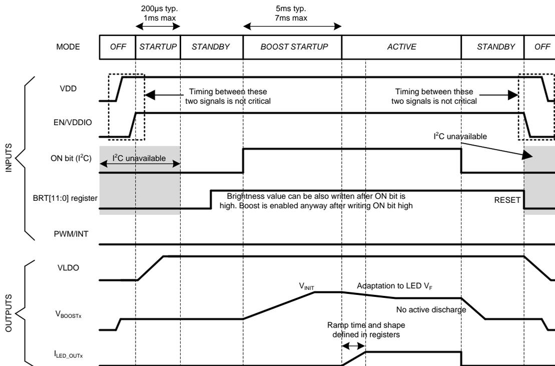
Figure 35. Start-up And Shutdown With I<sup>2</sup>C Brightness Control Mode (BRTMODE = 01b)
