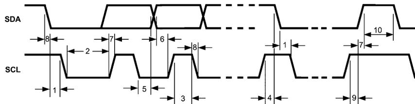
Figure 1. I<sup>2</sup>C Timing Parameters
