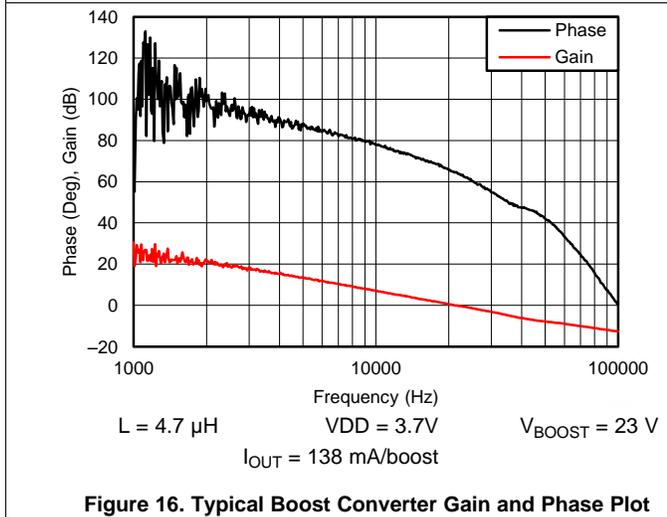
**Figure 16. Typical Boost Converter Gain and Phase Plot**
