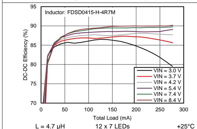
Figure 12. Boost Efficiency
